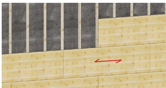
Structure verticale (mur) – pose horizontale
